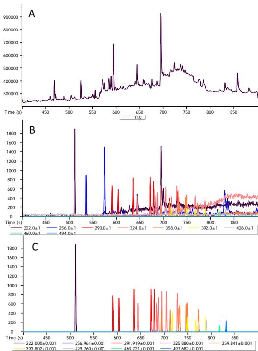
**Figure 6. Fish Oil + 100 ng/g PCB Standard - TIC (A), XIC at Unit Resolution (B), XIC at R = 25,000 (C).**
