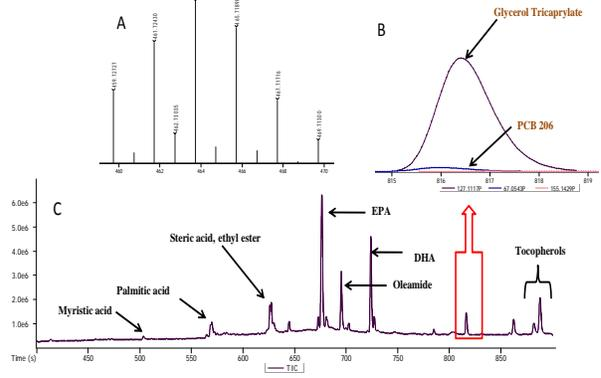
Figure 5. TIC of Fish Oil (C) Showing Coeluting Compounds Glycerol Tricaprylate and PCB 206 (B) and the molecular ion region of the mass spectrum for PCB 206 (A).
