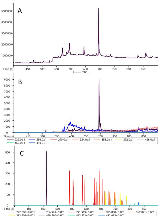
**Figure 7. Fish Oil + 10 ng/g PCB Standard - TIC (A), XIC at Unit Resolution (B), XIC at R = 25,000 (C).**
